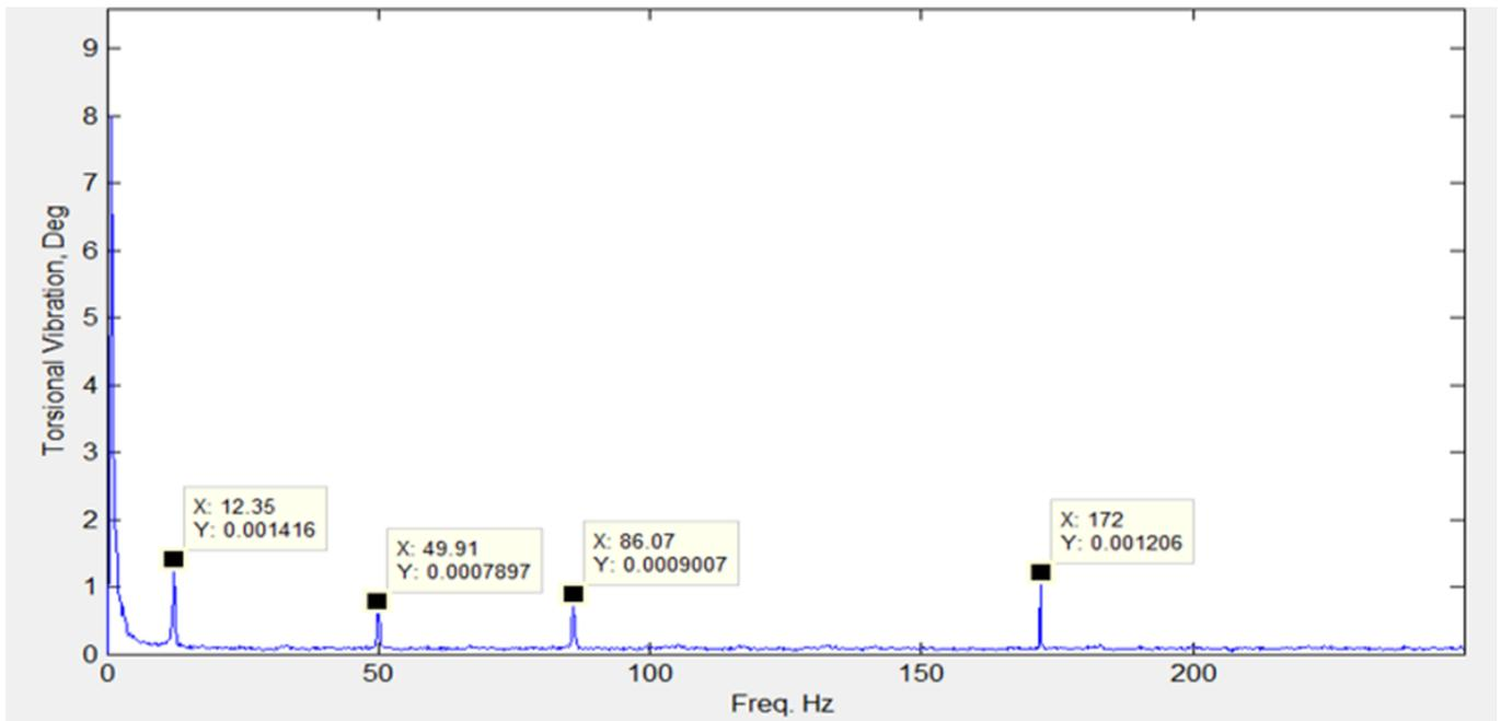
Figure 3: Torsional Vibration Analysis from Zebra Tape Encoders
