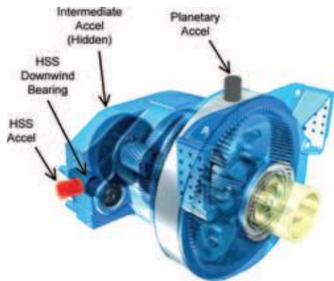
Figure 1: Wind turbine gearbox, viewed from the main rotor side. The high-speed shaft downwind bearing (HSS DW) and accel locations are shown. The high-speed accel location used for this case history is shown in red.
