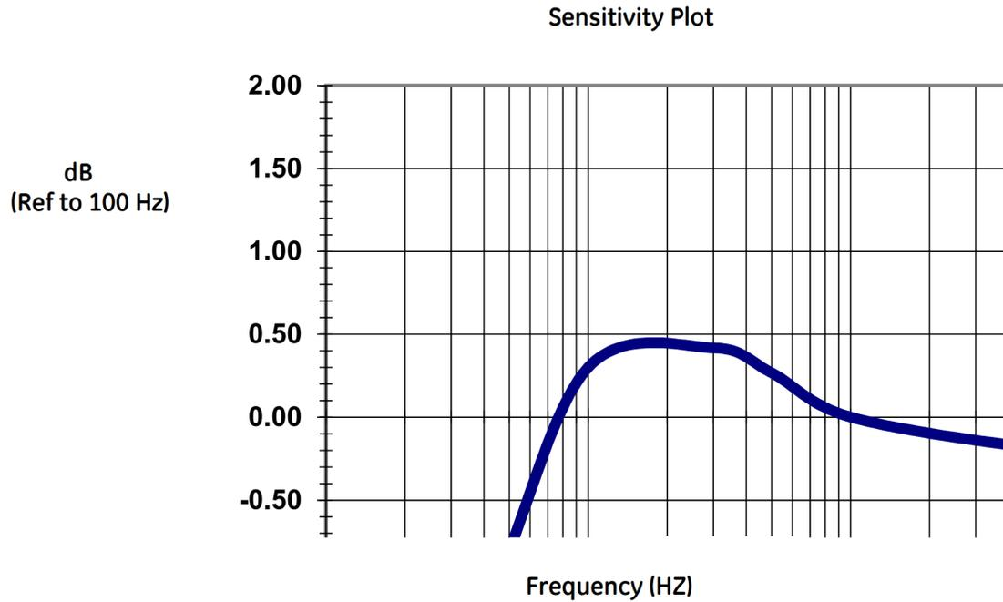
**Figure 2: Frequency Response, Typical Amplitude Response**
